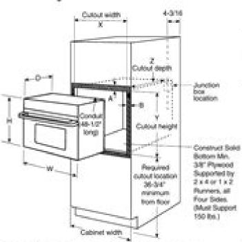
AnAllow 17 overlap of oven over top and bottom edges of output. Bu-Allow 15/36"-Self" for overlap of over-over side edoes of output.
