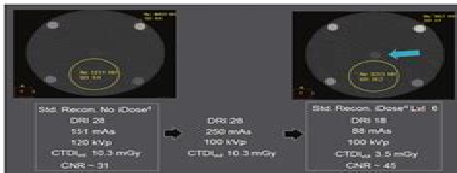
Figure 8 A 16 cm phantom with five iodine samples was used to show how the DRI can simplify adjustments in the tube potential, mAs, and iDose 4 . These adjustments lead to an increase in the CNR at low dose.
