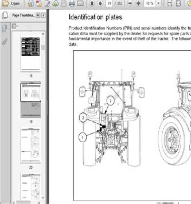
Product Identification Numbers (PIN) and serial numbers identify the tractor and its main components. The identification data must be supplied by the dealer for requests for spare parts or service operations. Identification data is of fundamental importance in the event of theft of the tractor. The following provides the locations of the identification
