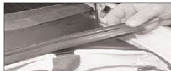
24.2 Pull off the rubber weatherstrip from the top of the bulkhead
