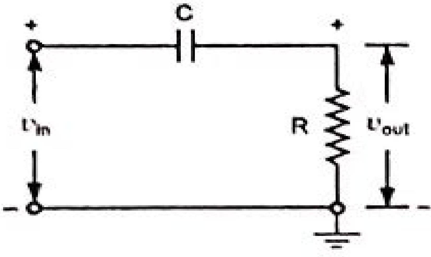
Fig. 29.1 *High-Pass R-C Circuit*
