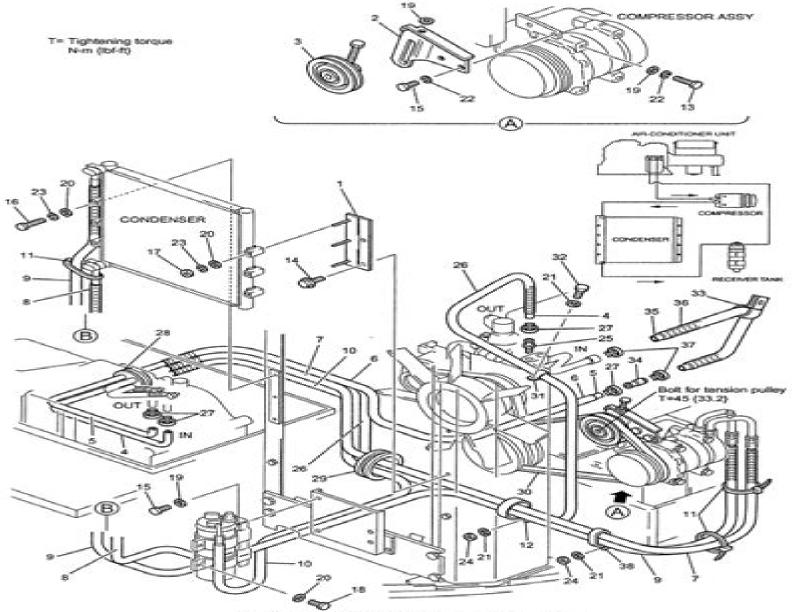
Fig. 25-2 Installing air conditioner and heater
