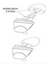
Align indicator lines on the ear tip and headphone nozzle for proper seal
