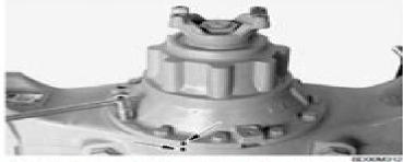
Put alignment marks on the differential carrier and axle housing. Remove 15 bolts securing differential carrier.
