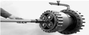
Pull the stub shaft out of the sun gear shaft. Be careful not to lose shim(s) that may be installed in sun gear shaft.
