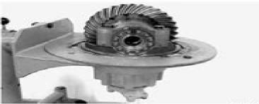
Mount differential carrier in OEM4135 engine stand using one CAS2847 holding bracket.
