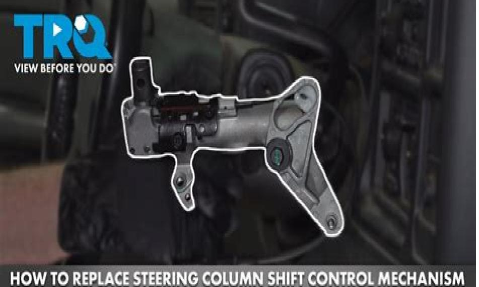
HOW TO REPLACE STEERING COLUMN SHIFT CONTROL MECHANISM 1999-2006 CHEVROLET SILVERADO
