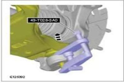
CAUTION: Do not use a hammer to separate the outboard CV joint from the hub. Damage to the threads and internal CV joint components can result.
