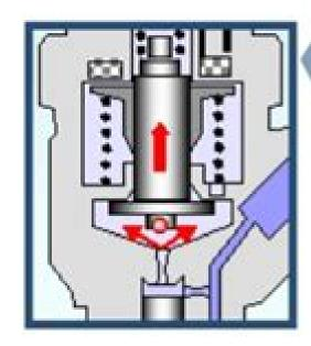
Maximum stroke of solenoid valve: approximately 50 micrometers (0.05 mm).
