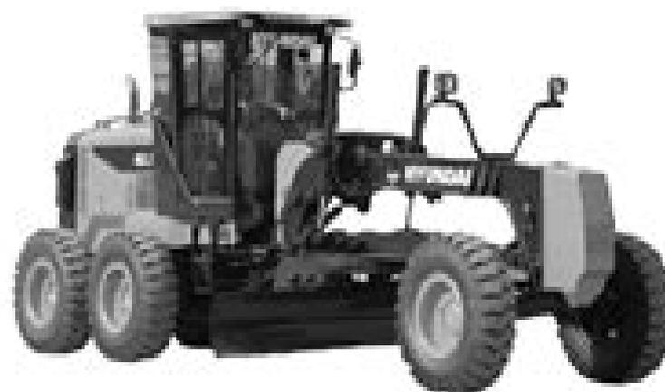
When traveling, set the blade at the maximum preparation angle and raise the blade fully.
