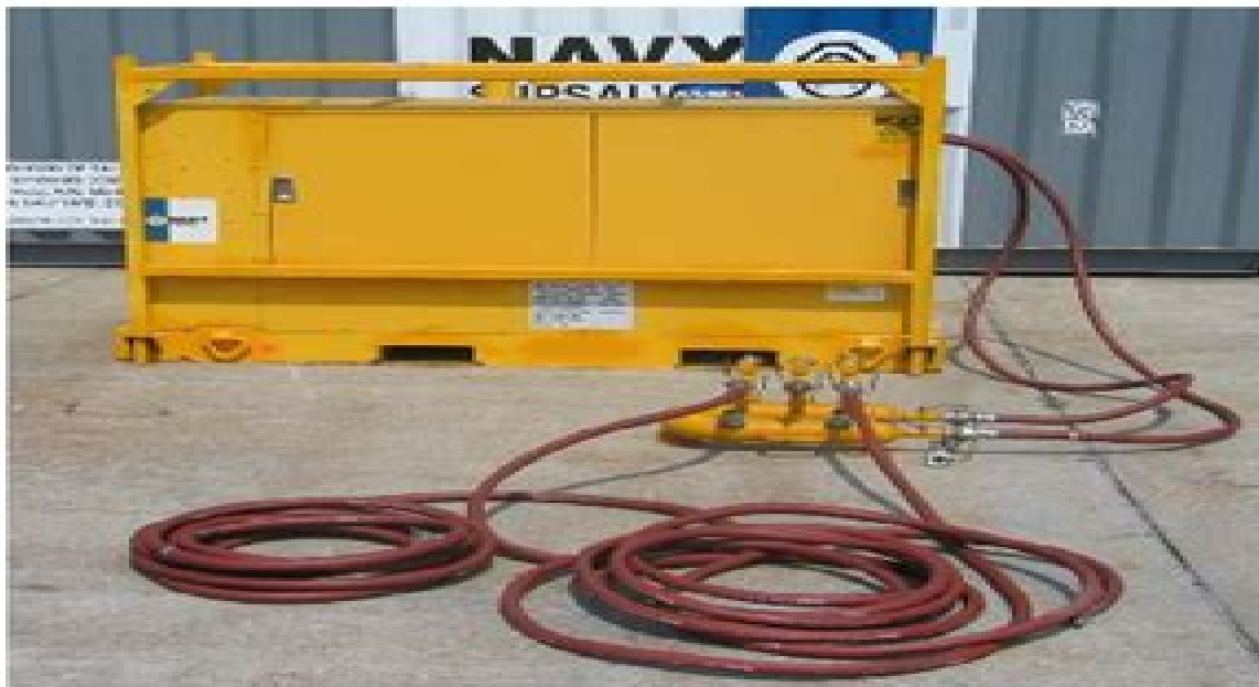
Overview of 175-Cfm Air Compressor System
