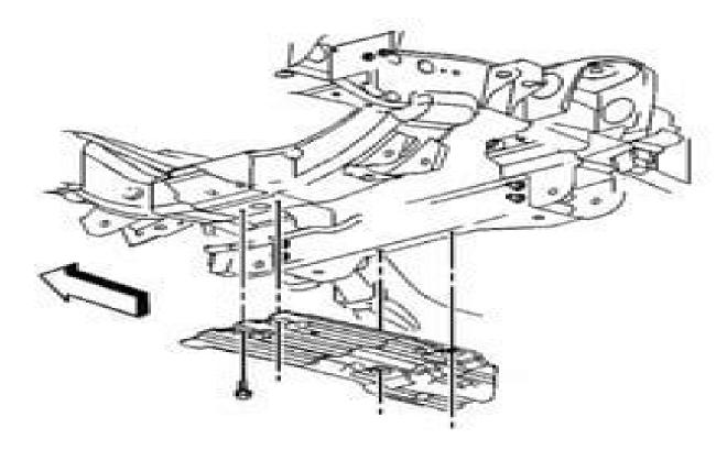
Fig. 1: Identifying Oil Pan Skid Plate Courtesy of GENERAL MOTORS CORP.
