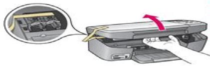
Lift the access door and remove tape inside the left side of the device.
