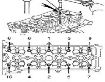
Cylinder Head Belt Torque Sequence
