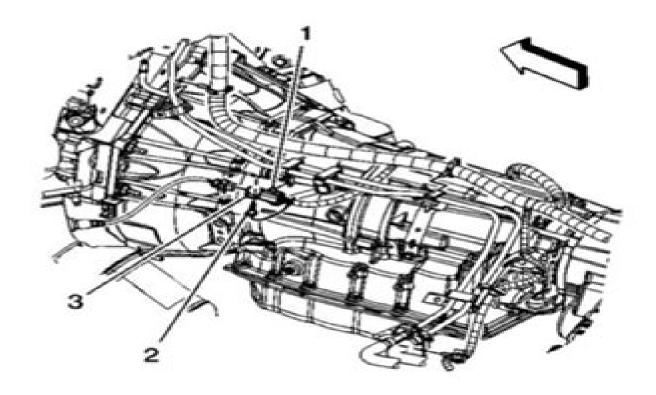
Fig. 17: View Of Engine Wiring Harness Electrical Connector Clip & Electrical Connector Courtesy of GENERAL MOTORS CORP.
