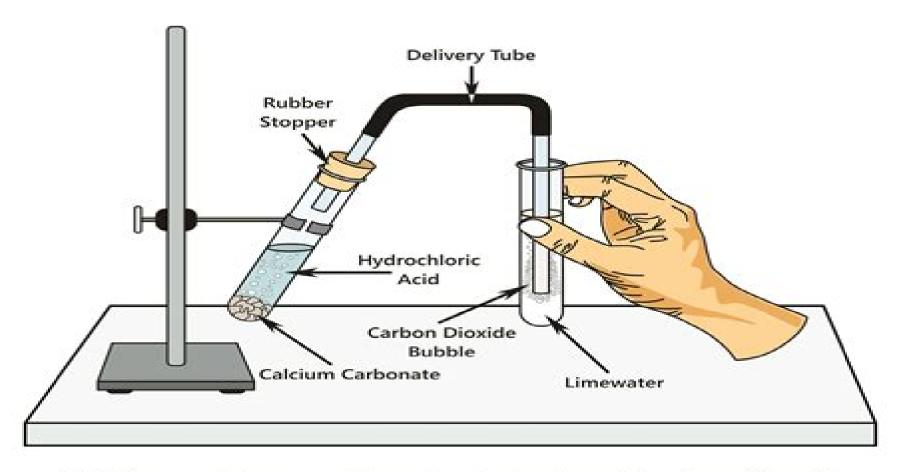
Adding calcium carbonate to hydrochloric acid will produce calcium chloride, carbon dioxide, and water.
