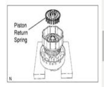
Place SST on the spring retainer, and compress the return spring with a press.
