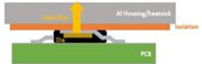
Top Cool concept method - Direct to heatsink
