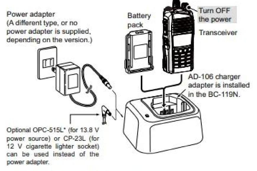
\*CAUTION: NEVER connect the OPC-515L to a power source using reverse polarity. This will ruin the battery charger.
