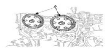
9 Remove the cam shaft.
