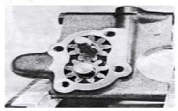
26. Remove the bolt 1 for the relief valve and check that the spring 2 and piston are in good condition. If there is anything suspicious about the opening pressure of the relief valve, check the data for the spring. See under "Technical Data, Lubricating oil pump". Clean and re-fit the piston and spring and tighten up the bolt.
