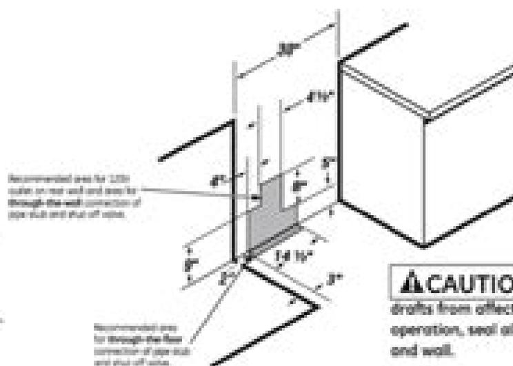
**CAUTION** To prevent drafts from affecting burner operation, seal all openings in floor and wall.
