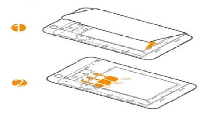
IdeaTab supports SD card and SIM card extension. To insert an SD card and SIM card , do the following:
