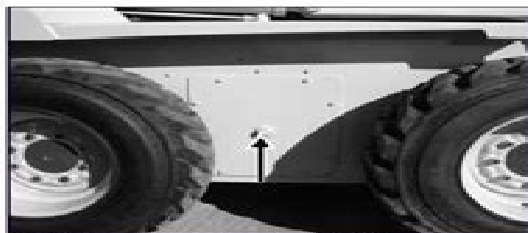
Fig. 3-9 Location of chaincase oil fill plug.
