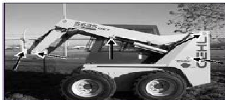
Fig. 3-10 Liftarm grease fitting locations.
