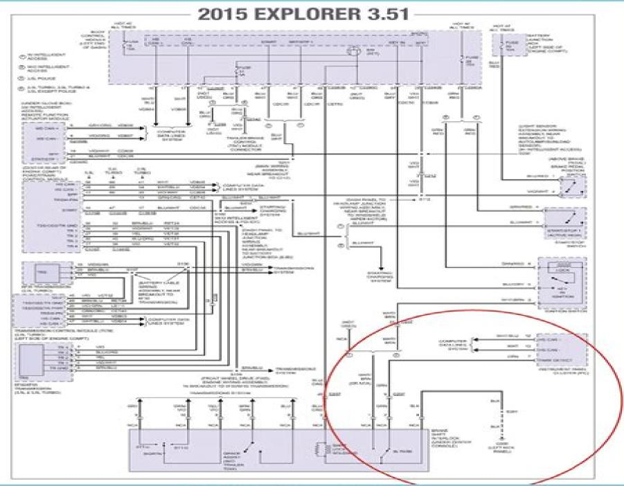
Figure 2: Shift Interlock System wiring schematic
