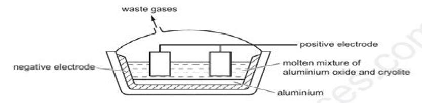
(i) Give two reasons why the electrolysis is done using a molten mixture of aluminium oxide and cryolite instead of molten aluminium oxide only.
