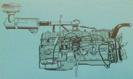
C-232 Gasoline Engine and Fuel System
