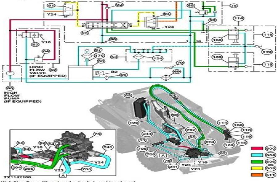
High Flow Pump (if equipped, wheeled machine shown)
