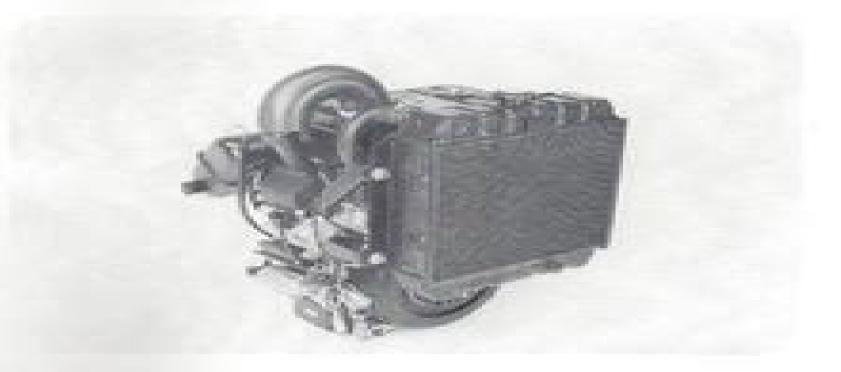
4-stroke liquid-cooled v-twin gasoline engine
