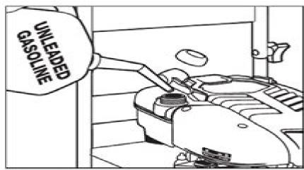
Step 3 Fill gas tank with unleaded gasoline. Do not use leaded gasoline.
