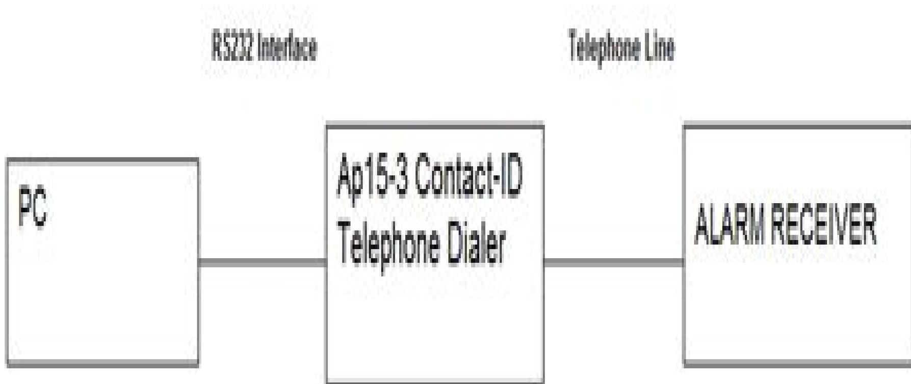
Popular alarm messages are originated at PC and sent to distant alarm receiver over telephone line.
