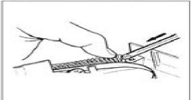
Press down the brake spring by means of a Phillips screwdriver.
