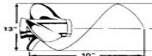
Diagram to explain the pitch dimension of a propeller. The pitch is the theoretical distance a propeller would travel through the water if there was no slippage.
