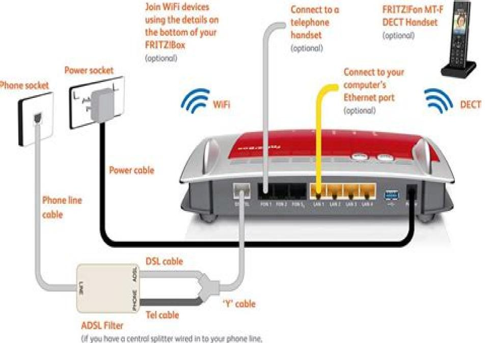
(if you have a central splitter wired in to your phone line, with a dedicated wall socket for DSL and your phone, connect the DSL and Tel cables directly to the wall sockets)
