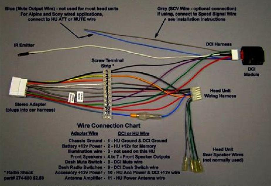
Note: This drawing shows an IR OCI, but the wiring is similar for all types of DCI's. Different HU brands may have different wire colors on the HU Wire Harness, so check your head unit manual before wiring.
