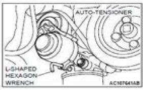
To reuse the drive belt, draw an arrow indicating the rotating direction (to the right) on the back of the belt using chalk, etc.
