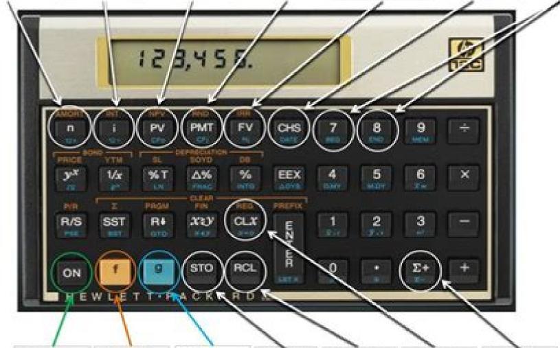
Power On/Offkey The orange if Function shift key, when pressed, activates the Orange versions of the various keys The blue g function shift key, when pressed, activates the Blue versions of the various keys
