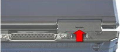
Turn the LifeBook up and use a plastic pry tool to release the Hinge Cover tabs on both sides.
