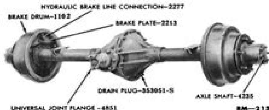
Figure 1— Standard Rear Axle Assembly
