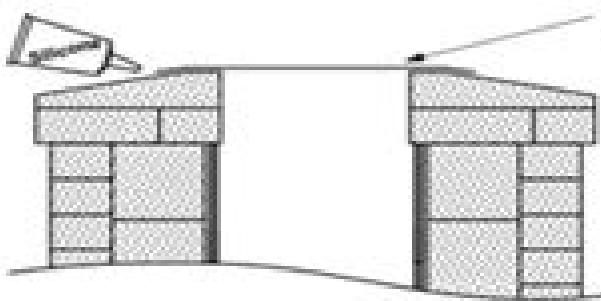
Cover plate is required if chimney does not have suitable rain cap.
