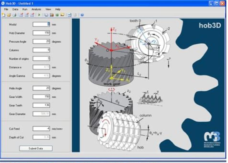
**HOB3D - CAD based Gear Hobbing Simulation**
