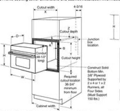
AnAllow 1" overlap of oven over top and bottom edges of cutout. 8inAllow 11/16"-3r4" for overlap of oven over side edges of cutout.
