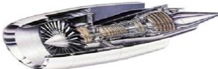
GE-90 TURBOFAN ENGINE (CUT-AWAY VIEW)
