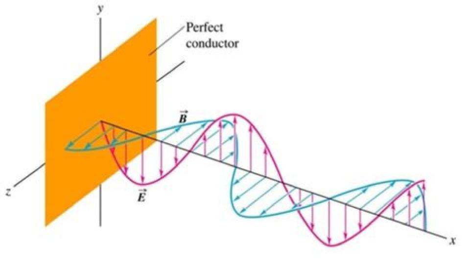
A standing electromagnetic wave does not propagate along the x-axis; instead, at every point on the x-axis the E and B fields simply oscillate.
