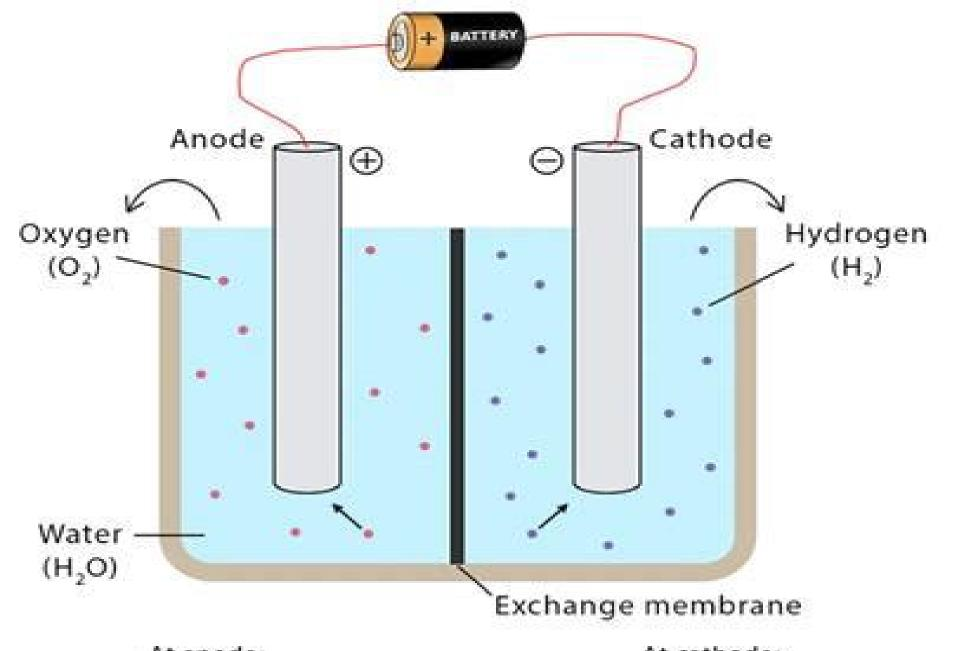
At anode: At cathode:  $2 \text{ H}_2\text{O (I)} \longrightarrow \text{O}_2(g) + 4 \text{ H}^{\oplus} + 4 \text{ e}^{\ominus} \qquad 2 \text{ H}^{\oplus}(\text{aq.}) + 2 \text{ e}^{\ominus} \longrightarrow \text{H}_2(g)$
