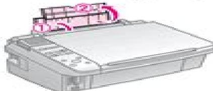
2. Open the output tray and slide out the extensions.
