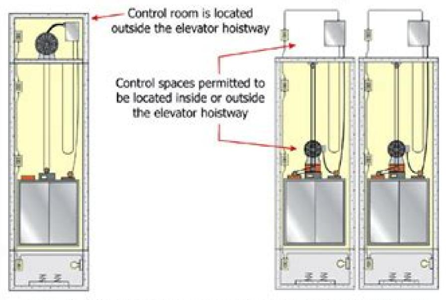
Article 620 defines spaces as well as rooms for elevator motor controller
