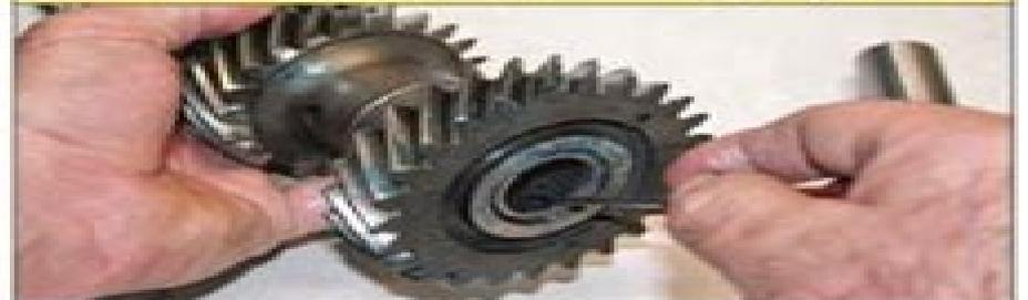
*You can use a small screwdriver to squeeze the needles together to check if you have room for a needle you may have left out. Again, this is something you cannot do with a dummy shaft.*
